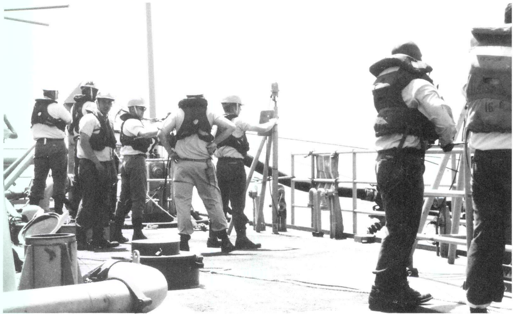
(above) Closing within 100 feet of this oiler, USS CURTS prepares to receive a refueling probe.
